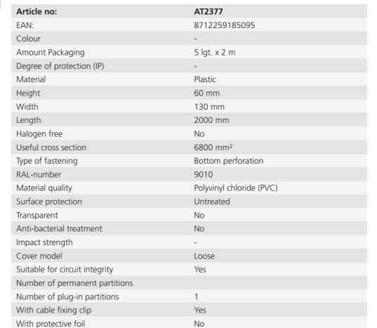
Attema Cable ducts KG are suitable for the well-organized installation of cables, for guiding heavy power cables or for the supply of power to high-quality computer equipment. The raceways have carefully thought out pre-punched holes for quick, precise positioning. Divider walls can be installed where necessary. All the raceways feature solid cover attachment and are available in a range of colours.
