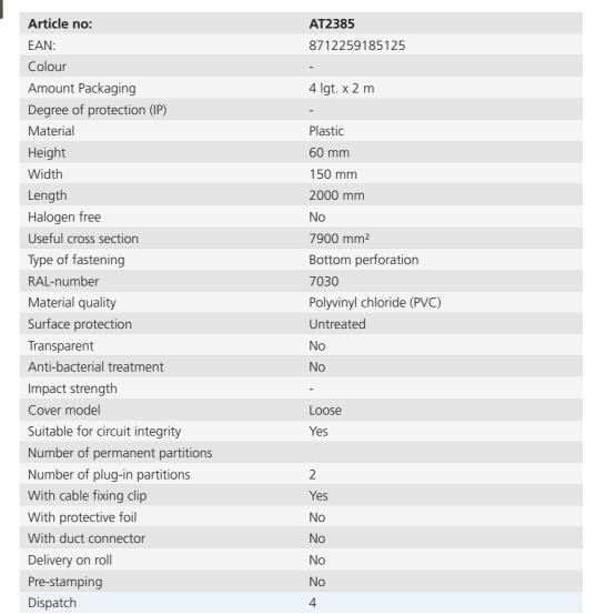
Attema Cable ducts KG are suitable for the well-organized installation of cables, for guiding heavy power cables or for the supply of power to high-quality computer equipment. The raceways have carefully thought out pre-punched holes for quick, precise positioning. Divider walls can be installed where necessary. All the raceways feature solid cover attachment and are available in a range of colours.
