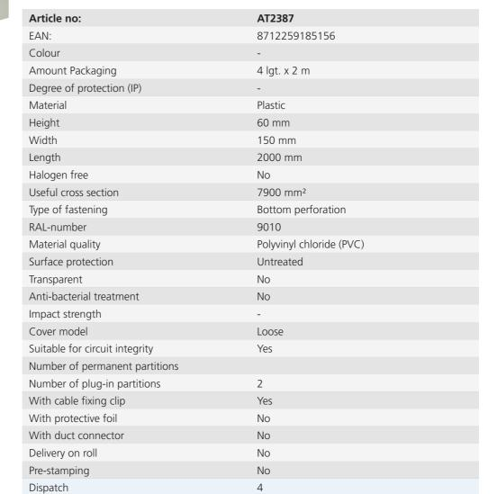
Attema Cable ducts KG are suitable for the well-organized installation of cables, for guiding heavy power cables or for the supply of power to high-quality computer equipment. The raceways have carefully thought out pre-punched holes for quick, precise positioning. Divider walls can be installed where necessary. All the raceways feature solid cover attachment and are available in a range of colours.
