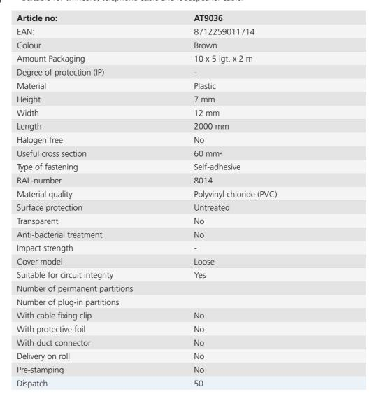
Attema raceways Z25 and KK are available in sizes ranging from small to large. Most mini-cable ducts are simple to install thanks to the high-quality double-sided tape. A number of raceways are available in various colours. Type TK does not have a cover. Type SK has a hinged cover with a secure closure. The MK10 consists of a raceway with a click-to-close cover.
