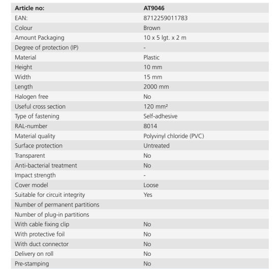
Attema raceways Z25 and KK are available in sizes ranging from small to large. Most mini-cable ducts are simple to install thanks to the high-quality double-sided tape. A number of raceways are available in various colours. Type TK does not have a cover. Type SK has a hinged cover with a secure closure. The MK10 consists of a raceway with a click-to-close cover.
